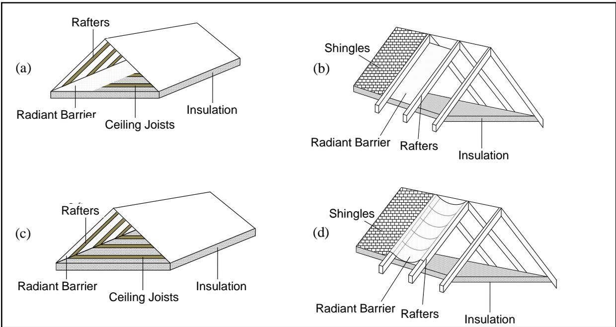
**Figure 1.** Common radiant barrier installation configurations: (a) horizontal radiant barrier (HRB), (b) truss radiant barrier (TRB), (c) deck-applied radiant barrier (DARB), (d) draped radiant barrier (DRB).
